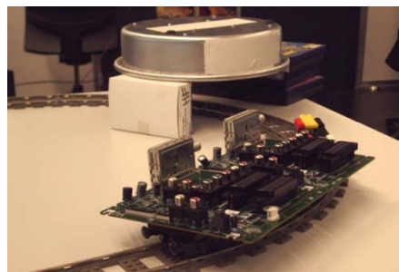
Test setup with Lego train, antenna above the board
